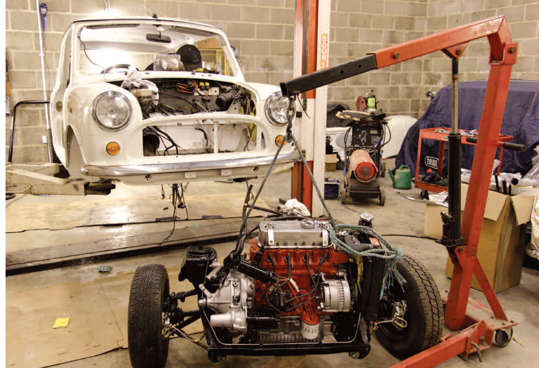
Full service! The mini's engine is removed from the shell at the Autocrash premises in Douglas.
